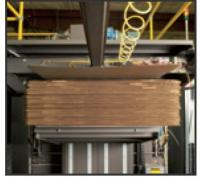
Optional Layer Sheet Placer: (1) Uses floor level magazine loading and (2) Vacuum picks all 4 corners of slip sheet for accurate placement.
