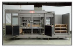
Design includes important safety features, such as a framed guard door package, CAT II safety circuits and muting light curtains. The CAT II safety meets the requirements of the most stringent safety programs. CAT III safety is also available as a low cost option.
