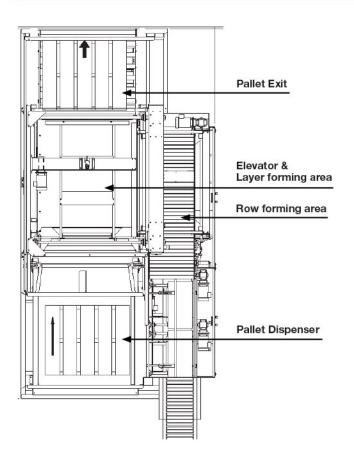
The new line of Currie by Brenton palletizers builds on more than six decades of experience building heavy-duty, reliable, easy-to-use palletizers. While offered at a modest cost, the LLP will provide many years of reliable service. With an install base of over 1,500 palletizers, many are still in operation after forty years of service.
