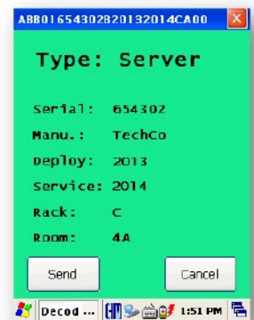
Fig. 2: Customized decoded data on valid Read
