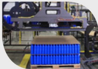
Robot moves to the pallet load position and lowers next layer level.
