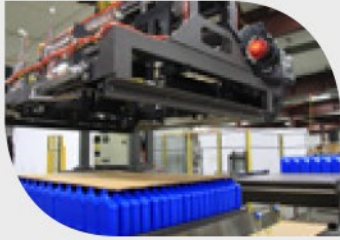
MasterPal™ tool then lowers over the formed layer on the pick table to capture the product. The internal tool clamping energizes to stabilize the product within the formed layer.
