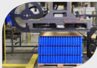
MasterPal™ tool slatted apron retracts to place formed layer atop the waiting pallet/lower layer. Then the clamping system retracts and the robot raises the tool above the pallet.
