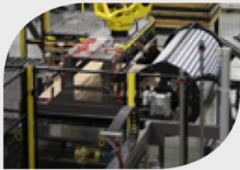
Robot moves to slide the product off the table end while the floor of the MasterPal™ tool moves simultaneously replacing the table with the floor of the tool until the layer is completely captured within the tool.
