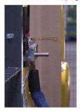
Corner boards are held to the load with beads of adhesive that are precisely sprayed on to the board. Customers can choose from a variety of adhesives to match their application.
