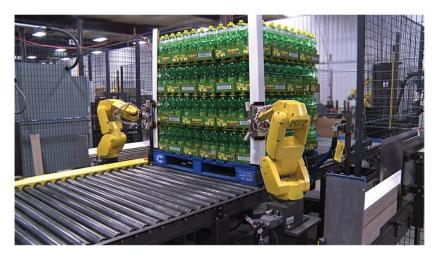
The Orion Robotic Corner Board Applicator places two corner boards at a time in the infeed area of the stretch wrapper. Customers who place cornerboards manually can realize substantial cost savings when upgrading to robotic corner board application.
