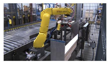
The Fanuc robot uses a specially engineered appliance to pick and place a variety of cornerboard types and sizes. Corner boards are loaded by operators outside of the Category 3 fencing and are then fed in to the production zone automatically.
