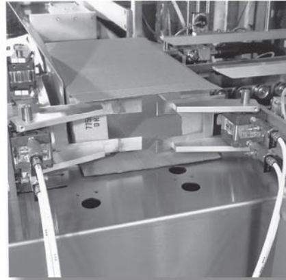
2. Back dust flaps are closed prior to product loading.
