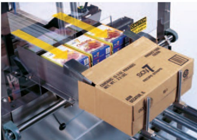
Product is automatically collated and loaded into the case
