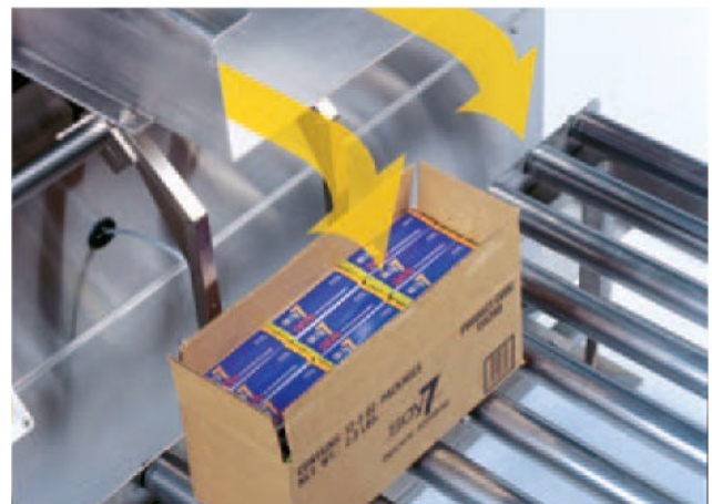
Loaded case is pneumatically lowered for discharge
