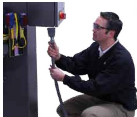
Operator simply plugs the cord from the new turntable base into the existing stretch wrapper
