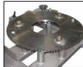
Turntable support on the Flex HPA provided by a precision ring bearing for maximum durability.
