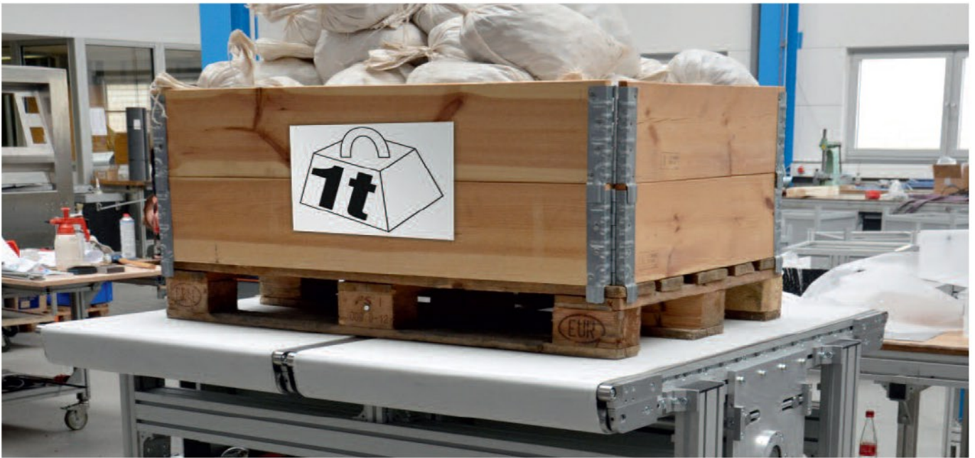
Belt Conveyor GUF-P 2041 with divided belt for loads to 1t
