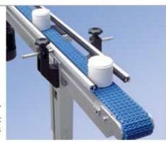
□ MBF-P 2040.02 Conveyor 90 mm wide modular plastic belt and adjustable side rails
