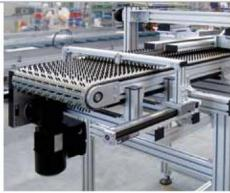
□ MBF-P 2040.02 Conveyor Special modular plastic belt with attachments
