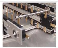
KTF-P 2010 Chain Conveyor Special attachment chain for transport of cam shafts
