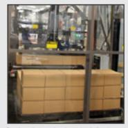
Product is received on the Infeed Conveyor at a 40" elevation. Product conveys to a stop and the Gantry lowers in position over the product on the conveyor.
