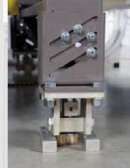
Conveyor Leg Load Cell
