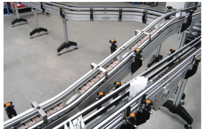
Flat top chain conveyor SBF-P 2254 with belt conveyor GUF-P 2000
