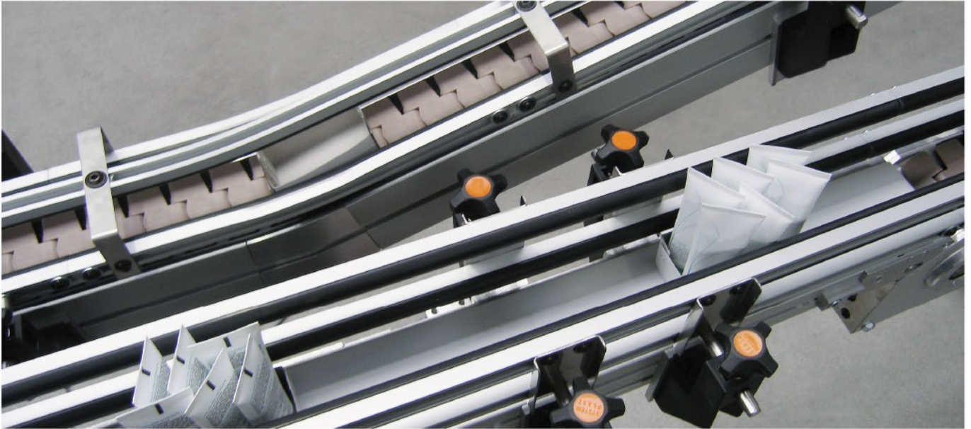
Flat top chain conveyor SBF-P 2254 with belt conveyor GUF-P 2000
