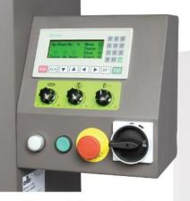
The control panel features a user-friendly display, knobs for turntable speed carriage speed and film tension, power light, start button, E-stop button and power disconnect.
