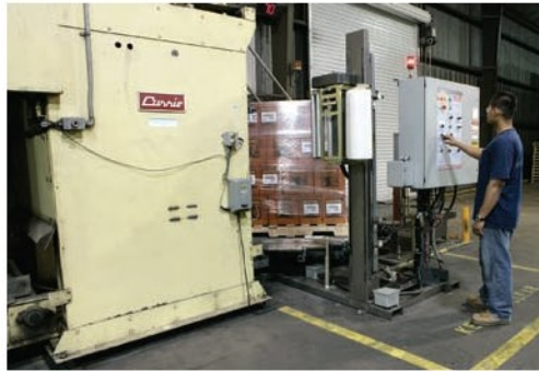
High level Currie palletizer mated with an Orion FA Series automatic stretchwrapper
