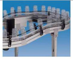
SBF-P 2254 Conveyor Table top chain conveyor with incline and transfer module
