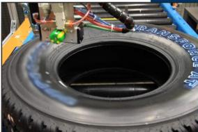
The robot paints only the decorative area of the tire. Continuous cell throughput is achieved by calculating the spray gun path on one side as the robot paints on the other lane.
