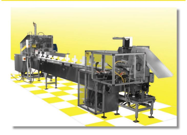
A completely automatic system for forming, conveying, closing and sealing top loaded cartons.
